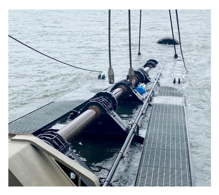
Safe working pneumatic actuators are managing every situation whenever the dredging boom is above or below water.
